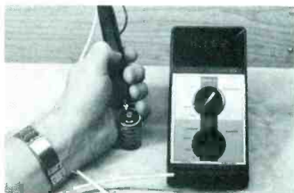
Fig. 9 The press-to-read probe with a sharp point is convenient for one-hand operation without the danger that slipping might cause shorts.
